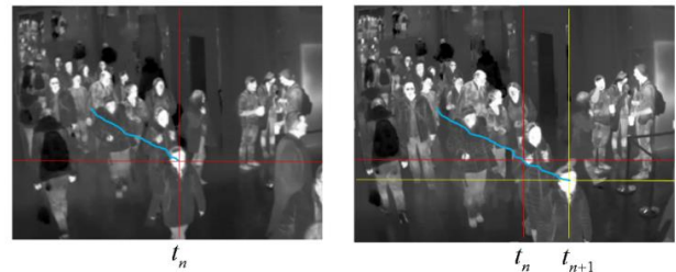
Figure 2. Pedestrian position in t_n and the next frame he/she is in next position t_{n+1} , the blue line is the virtual trajectory.
