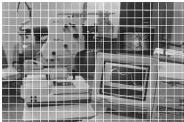
Figure 13. Image and grid used for the simulations of the optical distortion model.
